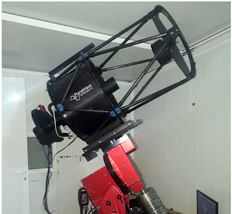
Figure 1. Maxim Usatov's 0.43m A1 telescope, a PlaneWave Corrected Dall-Kirkham (CDK) optical design equipped with the latest-generation back-illuminated Sony IMX455 sensor and located at a remote site in Spain.
